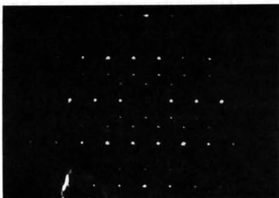
Fig. 3. Typical observed [100] electron diffraction pattern of a hollandite.
